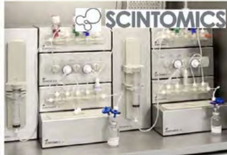
Two GRP Cassette Systems in one Hot Cell
